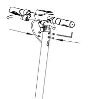
2: Fasten the front tube and the folding stem with the hex wrench and screws.
