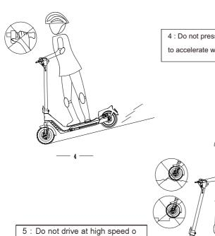
4 : Do not press power throttle to accelerate when going downhill.
