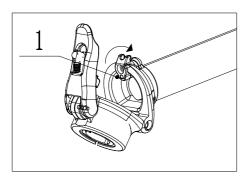
When riding for a period of time and feel that the gap between the folding stem is too large, you can use tools to adjust the folding mechanism on the folding seat.
