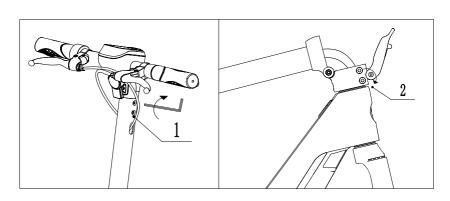
When you feel the front tube of the scooter is shaking, please use a 2.5MM hex socket tool to tighten counterclockwise the four screws at the joint between the front tube and the stem (position 1). Tighten counterclockwise the two screws of the stem base with a 5MM hexagon socket. (position 2)
