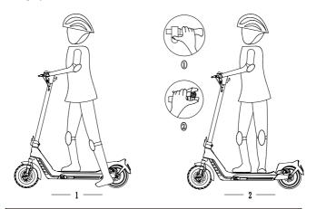
1: The scooter need a kicking off starting. When power is on, one foot stands on the pedals and the other foot kicks back on the ground. 2: When the scooter is sliding, then the other foot back on the pedals. When the scooter is stable, then push the right power throttle. ①. Hold left hand on the brake lever tightly when braking. ②. Front wheel drum brake and rear electronic brake is in effect simultaneous.
