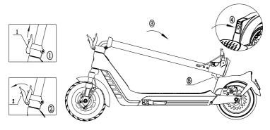
When folding, turn off the power, first lift up the safety lock, then open the safety lever, then fold the folding stem to the rear part of the scooter. Lift the hook buckles on the rear mud guard, and finally buckle the 2 hooks together to complete the folding.
