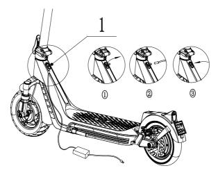
The charging port is located at position "1" on the front right side of the scooter. When charging, firstly open the dust-proof cap, and then insert the charging port. When the indicator light is red, it means charging is in progress. When turns green, charging is complete. Finally unplug the charging port and fasten the dust-proof cap.
